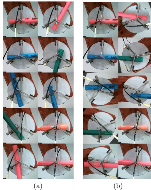
Figure 16: Orientation correction: (a) Random subset of successful grasps (b) Images of the grasps have been rotated based on their estimated orientation in order to orient the marker horizontally.
